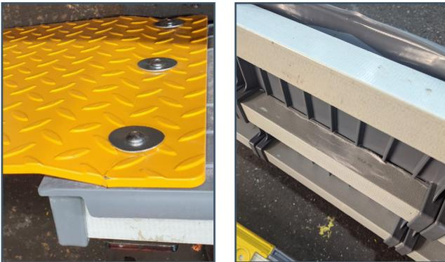
Examples of damage shown above; bent steel plates, left, and cracked structural sections, right. This list is not exhaustive
