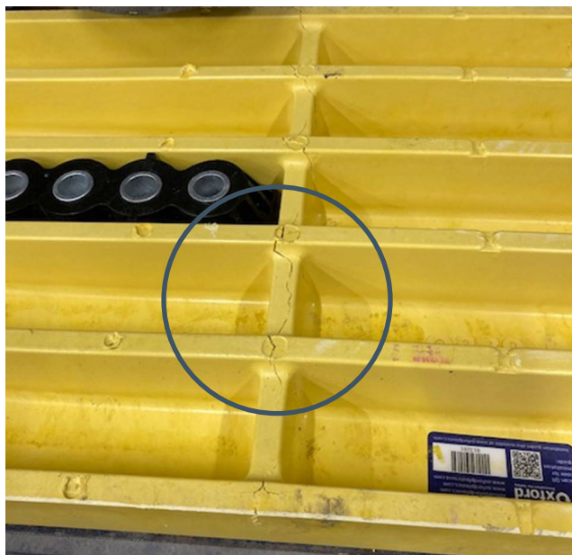
Crack along rib
